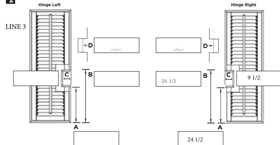
**Notes:** Cut outs are rectangular: Standard dimensions = 10" inside cut out in height and 5" inside cut out in depth.
